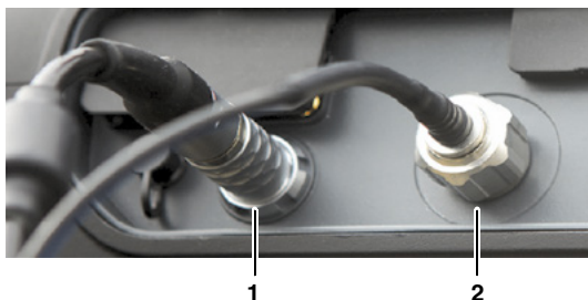
Figure 3: Connecting RF cable: Control connection (1) and N connection (2)
