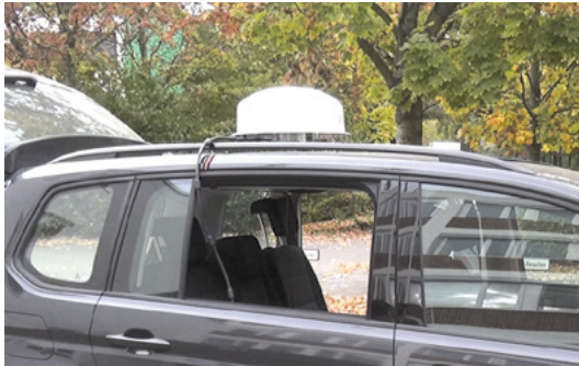
Figure 6: Mounted ADFA with security strap and routed RF cable.
