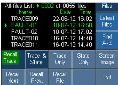
Files are stored under either default file names, or user-chosen file names entered from an alpha-numeric keypad.
