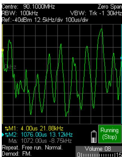
In addition to audio demodulation of AM or FM signals, the modulating waveform can be displayed against a timebase settable between 5µs/div and 20ms/div.
