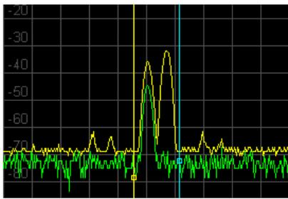
When in Peak-hold or Average modes, dual display traces can be selected enabling the processed and unprocessed traces to be seen simultaneously.
