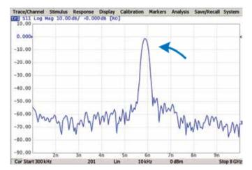
This function performs data transformation from frequency domain into response of the DUT to various stimulus types in time domain. Modeled stimulus types: bandpass, lowpass impulse, and lowpass step. Time domain span is set by the user arbitrarily from zero to maximum, which is determined by the frequency step. Windows of various forms are used for better tradeoff between resolution and level of spurious sidelobes.
