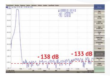
Typical dynamic range of 123 dB is achieved from 300 kHz through the top of the frequency range (at 10 Hz IF bandwidth). Seen here is the maximum dynamic range achieved when using IFBW 1 Hz and an output power level of 5 dBm.
