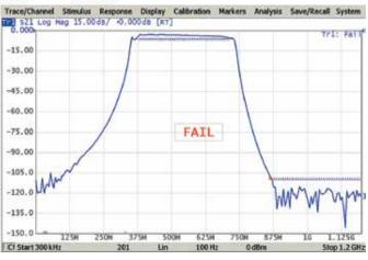
Limit testing is a function of automatic pass/fail judgment for the trace of the measurement results. The judgment is based on the comparison of the trace to the limit line set by the user and can consist of one or several segments.
