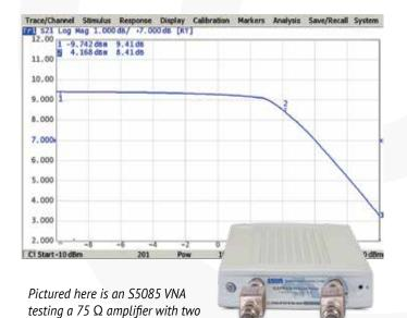
The power sweep feature turns compression point recognition, one of the most fundamental and complex amplifier measurements, into a simple and accurate operation.
