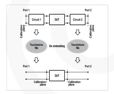
This function allows the user to mathematically exclude the effect of the fixture circuit connected between the calibration plane and the DUT from the measurement results. This circuit should be described by an S-parameter matrix in a Touchstone file.
