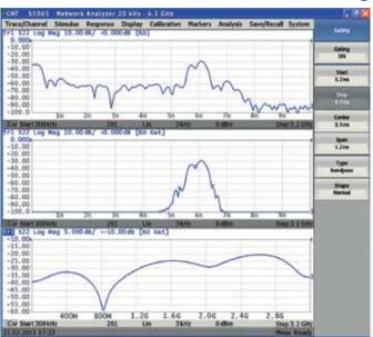
This function mathematically removes unwanted responses in the time domain, which allows the user to obtain frequency response without influence from fixture elements.
