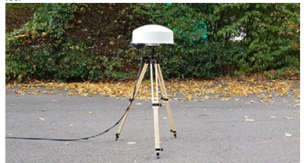
Fig. 4: Tripod - Semi-static operation, quick and easy to install
