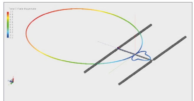
Fig. 9: Antenna 2 - Typical horizontal characteristic of the directional dipole antenna, computed for the far field.
