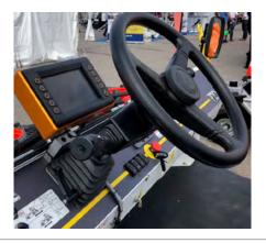
Real time load forces display on the auto brightness screen during the tow.
