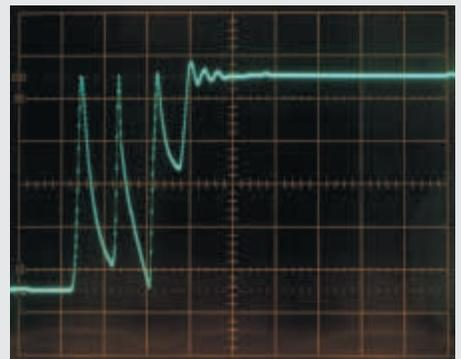
Arbitrary waveform - simulated contact bounce.
