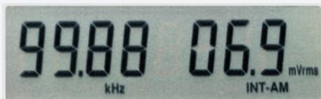
The decimal point and units are changed automatically resulting in a display of the true amplitude regardless of the attenuator setting.
