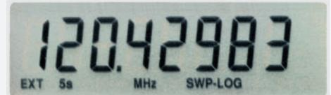
A measurement period of 0.5 or 5 seconds can be selected. A reciprocal counting measurement system is used which ensures high resolution regardless of input frequency.
