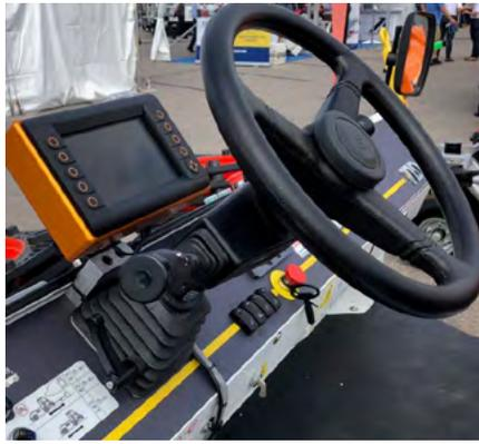
Real time load forces display on the auto brightness screen during the tow.
