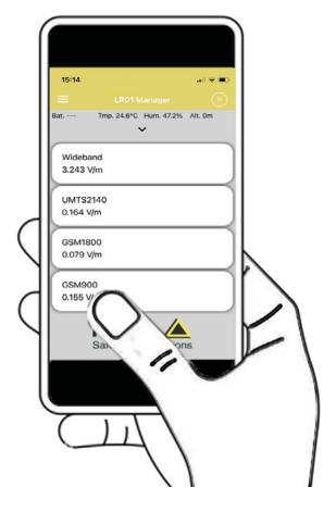
The app works with SMARTS AMC by Bluetooth connection so users can enjoy hands-free operation and stay at a safe distance from the potentially dangerous field. The user can easily display EMF measurements, browse the technical data (battery level, altitude, etc) and change settings by simply tapping the screen.
