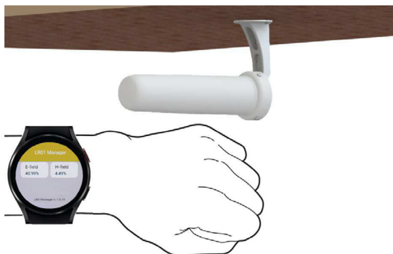
Fig. 2-7 AMC link with Bluetooth communication by smartwatch
