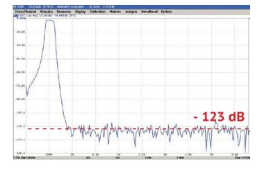
Typical dynamic range of 123 dB is achieved through the entire frequency range (at 10 Hz IF bandwidth). Seen here is the maximum dynamic range achieved when using IFBW 10 Hz and an output power level of 5 dBm.
