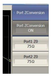
This function converts the S-parameters measured at the 75  $\Omega$  port into values, which could be determined if measured at a test port with arbitrary impedance.
