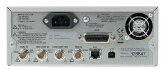
Rear panel mounts the digital interfaces and the rear I/O connectors. (Note: GPIB interface is only fitted to suffix G models)
