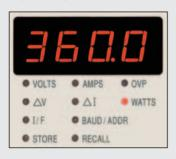
All keyboard entries appear on this display for inspection before they are actioned by pressing the "confirm" key.
