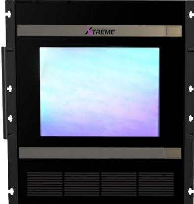
The **XTREME 256** defines the *next generation of L-band matrix switching systems featuring 256 ports in a compact 12 RU chassis*. The system is a full fan-out, non-blocking L-band RF Matrix Switch, whereas any input can be routed to any or all outputs.
