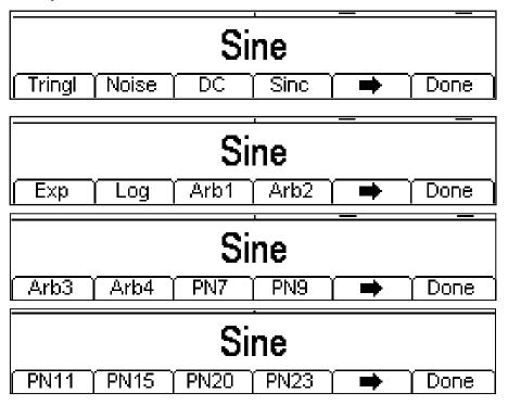
One more press of the soft-key will show the first list again. Select the modulation shape required by pressing the appropriate key then press the **Done** soft-key to return to the top level modulation menu.
