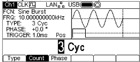
The count may be changed in either of the ways detailed in Numeric Editing Principles. The carrier waveform in the Graph Box will show a representation of the burst as the count is edited.
