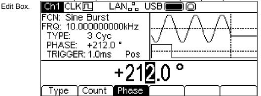
The phase may be changed in either of the ways detailed in General: Numeric Editing. The carrier waveform in the Graph Box will show a representation of the carrier start phase as the phase is edited. Note that the phase may also be set by pressing the **Phase** soft-key from the carrier menu.
