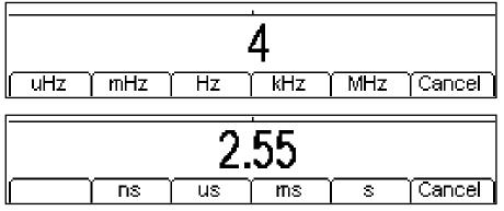
During the numeric data entry a decimal point and, if appropriate, a sign may be entered. The +/- key is used to alternately change the sign between + and –. The left cursor key may be used to erase the last digit entered. The entry may be cancelled by pressing the **Cancel** key
