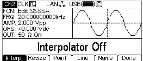
While editing an arbitrary waveform it will be available at the MAIN OUT connector of the selected channel for display on an oscilloscope. There is also a representation shown in the Graph Box and the FCN field in the Parameters Box shows Edit ARBNAME as a reminder that this waveform is temporarily selected for output.
