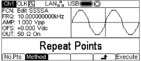
When a waveform is increased in size new points are added between existing points. The way that the values of these new points are calculated depends on the resize method setting, The **Repeat Points** method adds points of the same value as the original point in the waveform. The **Interpolate** method draws a straight line between the existing points.
