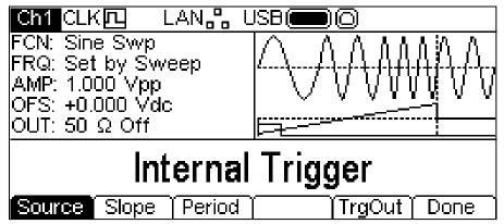
Repeated presses of the **Source** key will cycle round the four possible trigger sources: **Internal Trigger** (using the internal trigger generator), **External Trigger** (using the signal at the TRIG IN connector), **Manual Trigger** (from the Trigger key) and **Channel 2 Trigger Outout**. Internal Trigger also has **Slope** and **Period** keys, External Trigger and Channel 2 Trigger Output have only a **Slope** key and Manual Trigger has no additional keys.
