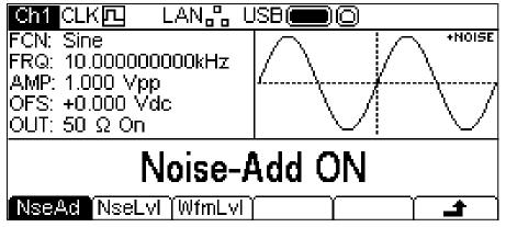
Pressing the **NseAd** soft-key will alternate between **Noise-Add ON** and **Noise-Add OFF**. With noise added the Graph Box shows **+NOISE** in the top right corner and two extra soft-key labels appear, **NseLvl** and **WfmLvl**.
