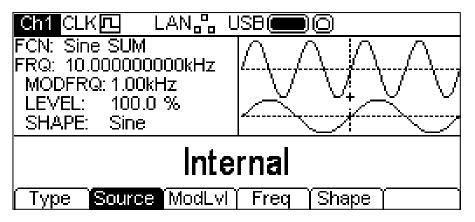
To select the modulation source press the **Source** soft-key. The options are **Internal** or **External**. Internal will use the waveform specified in the shape parameter and the Graph Box will show that shape as the modulating waveform. External will use the signal present at the MOD IN connector and the **Freq** and **Shape** soft-keys will disappear. The Graph Box will always show a sinewave as the modulating waveform if the source is set to External.
