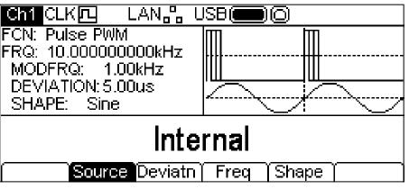
Note that PWM is the only modulation type applicable to pulse so there is no  $T_{ype}$  soft-key to allow selection of any other type.
