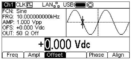
The offset may be changed in either of the ways detailed in General: Numeric Editing. During a new offset entry the +/- key can be used at any time to set a negative offset; alternate presses toggle the sign between + and -.
