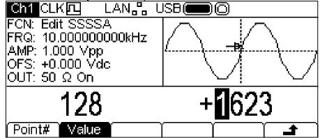
The point edit menu allows individual points in the waveform to be set to any vertical level value. The **Point#** soft-key selects setting of the point number; pressing the **Value** soft-key then enables the value to be changed. The point number and point value may be changed in either of the ways detailed in General: Numeric Editing. The point which is being edited is shown in the Graph Box by an arrow and a **x**. The point value is changed in the actual waveform immediately it is edited.
