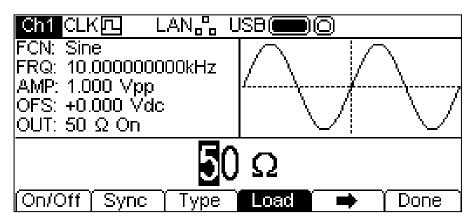
This is the value that is assumed to be loading at the instrument MAIN OUT connector. The value is used to calculate the actual values of amplitude and dc offset. Note that the output impedance of the instrument MAIN OUT connector is fixed at  $50\Omega$ .
