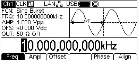
Notice that **Burst** still shows in the **FCN** field of the Parameters Box and the BURST key still glows yellow indicating that burst is still active. To return to the Burst menu to edit the burst parameters press the BURST key again. To turn off burst press the BURST key while the Burst menu is displayed.
