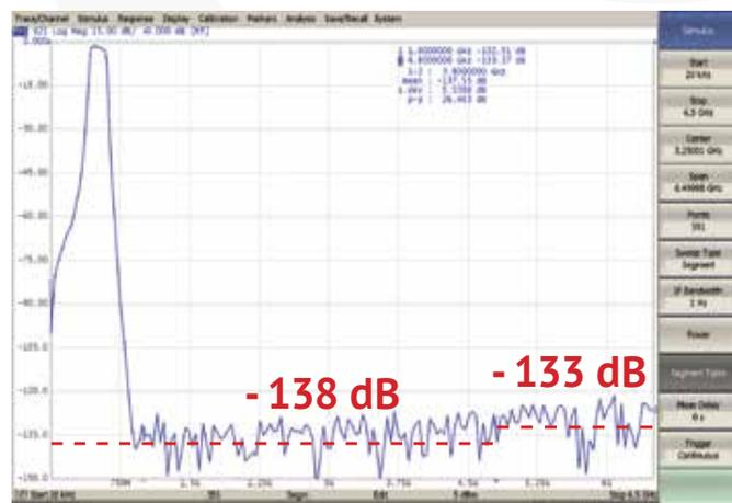
Typical dynamic range of 123 dB is achieved from 300 kHz through the top of the frequency range (at 10 Hz IF bandwidth). Seen here is the maximum dynamic range achieved when using IFBW 1 Hz and an output power level of 5 dBm.
