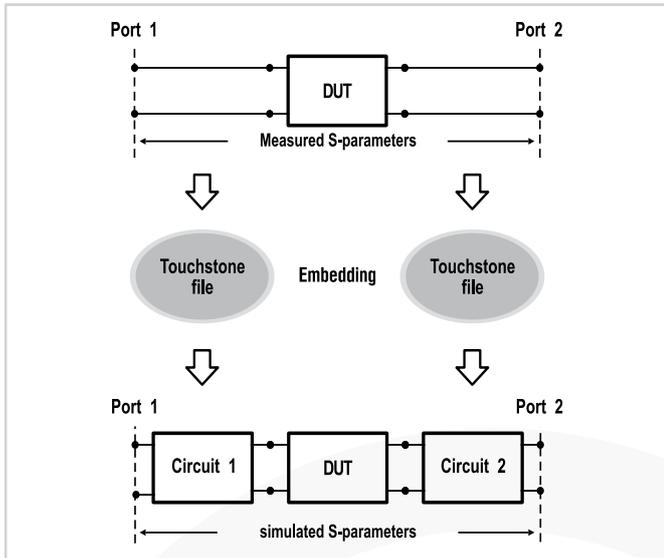
This function allows the user to mathematically simulate DUT parameters by virtually integrating a fixture circuit between the calibration plane and the DUT. This circuit should be described by an S-parameter matrix in a Touchstone file.
