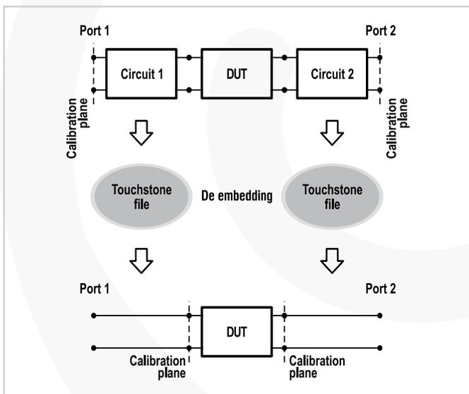
This function allows the user to mathematically exclude the effect of the fixture circuit connected between the calibration plane and the DUT from the measurement results. This circuit should be described by an S-parameter matrix in a Touchstone file.
