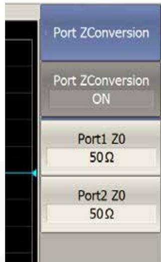
This function converts the S-parameters measured at the 50 port into values, which could be determined if measured at a test port with arbitrary impedance.
