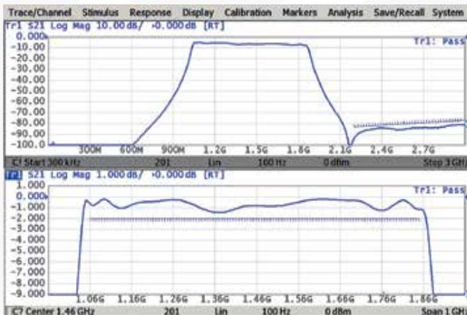
Limit testing is a function of automatic pass/fail judgment for the trace of the measurement results. The judgment is based on the comparison of the trace to the limit line set by the user and can consist of one or several segments.
