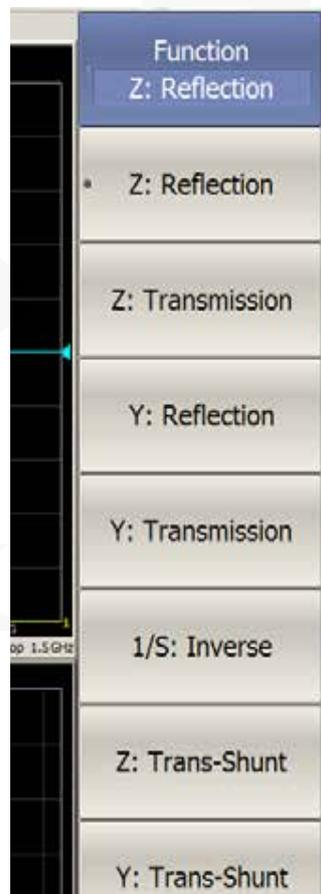
The function allows conversion of the measured S-parameters to the following parameters: reflection impedance and admittance, transmission impedance and admittance, and inverse S-parameters.
