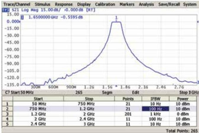
The VNA has a large frequency range with the option of frequency scan segmentation. This allows optimal use of the device, for example, to realize the maximum dynamic range while maintaining high measurement speed.
