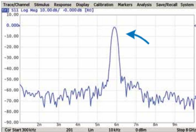
Here, built-in time domain analysis allows the user to detect a physical impairment in the antenna feeder.
