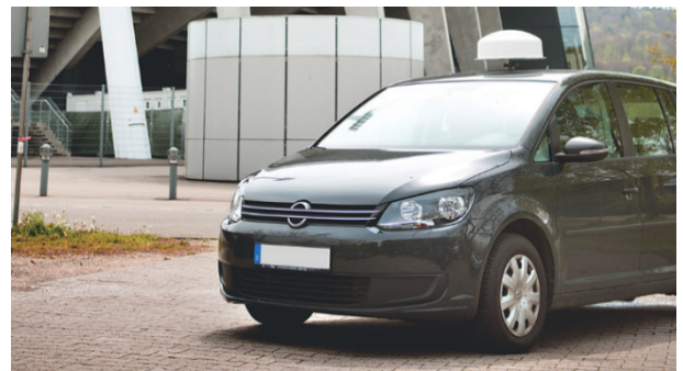
Magnetic mount: Non-destructive, fast mounting on a vehicle roof
