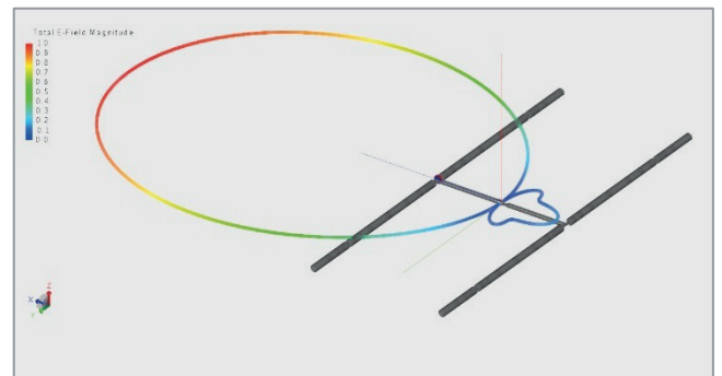
Antenna 2: Typical horizontal characteristic of the directional dipole antenna, computed for the far field.
