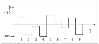
Fig. 7. Example of a phase angle pattern.
