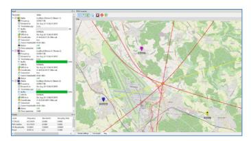
Fig. 1. Example of a localization based on a hybrid system realized by Narda SignalShark Receivers and Decodio Localizer Software.
