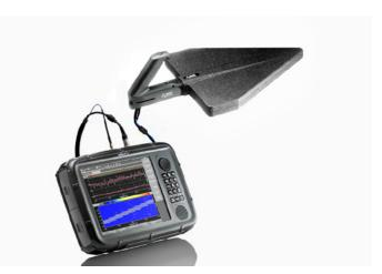
Fig. 10. Narda SignalShark now equipped with a manual antenna for homing purpose.
