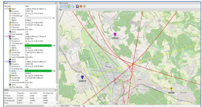
Fig. 1. Example of a localization based on a hybrid system realized by Narda SignalShark Receivers and Decodio Localizer Software.
