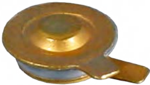
The example to the left is a 4BT-2 configuration, open on rise, silver contacts, open on rise at 41°C ± 4.4°C, close at 24°C ± 4.4°C with 12" wire leads
