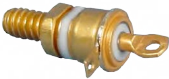
The example to the left is a 3BT-6 configuration, close on rise, gold contacts, close on rise at 82°C ± 4.4°C, open at 65°C ± 4.4°C.
